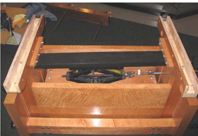
With top removed, jack mechanism is visible. Notice the book matched tiger maple of the frame.
