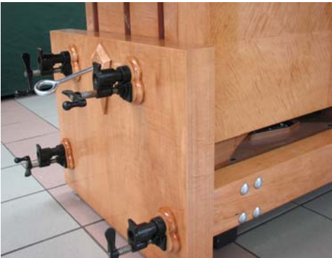
Loosen pipe clamps and turn eyelet with jack handle
