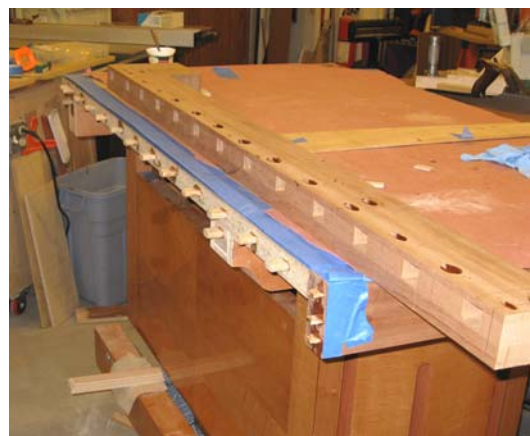
Top edging ready for glue up Festool used to make 18 loose tenons
