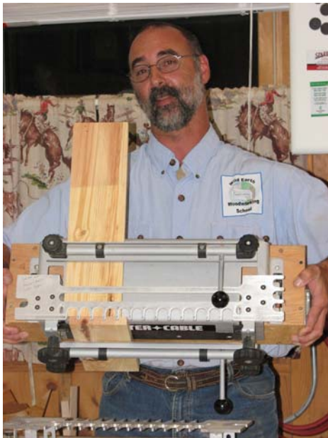
Fixed finger jig setup ready to cut Tails/pins will be cut at same time
