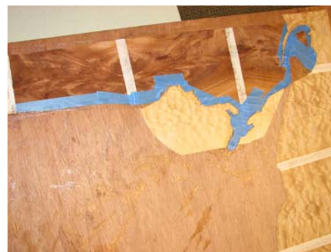
Plywood back ready for state inlays blue tape is for glue control
