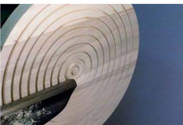
7. Layout alternating 3/8" wide beads and coves separated by 1/8" wide fillets. Cut fillets 3/16" deep.
