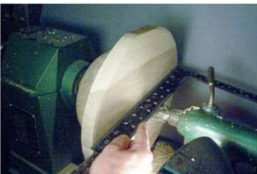
5. Check that each side is flat. Use sanding pad with course paper for final surfacing.
