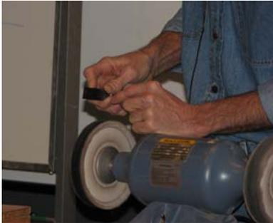
Then use a buffing wheel to produce the final cutting edge. The buffer to use is preferably a slower speed grinder/buffer. A grinder turns toward you with significant guards over the stone. A buffer turns away from you, usually without guards over the buffing wheel. A buffing wheel will not cut until it is dressed with a compound. Use an emery buffing compound. This is one of the coarsest of the buffing compounds.
