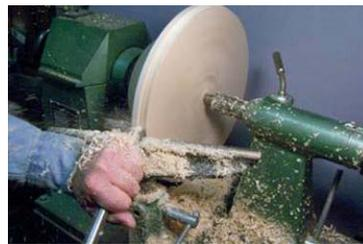
6. Secure blank to face plate with paper-glue joint. True-up disk edge to round.
