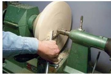
4. True-up one side of blank. Sand off small nubbin where blank is held by the tail stock. Reverse and true-up other side.
