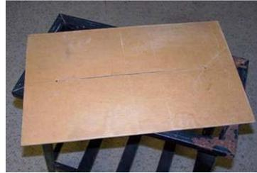
12. Slotted support table to allow piece to be assembled to final shape. Mark a line on rear face of the piece, to aid in reassembly.
