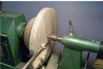
3. Trap blank between faceplate and tail stock with firm tail stock pressure. Start lathe slowly and assure blank is secure.
