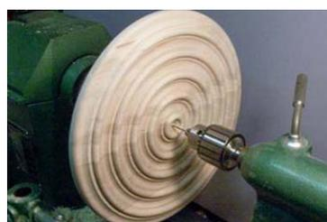
8. Turn beads and coves. Finish sand and seal front face. Drill small pilot hole through the disk, to mark center. Pry piece from drive faceplate with wood chisel.
