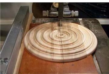
9. Make carrier board, guided by band saw fence. Cut turned piece on center along wood grain. Sand cut edges and make each half equal in size.
