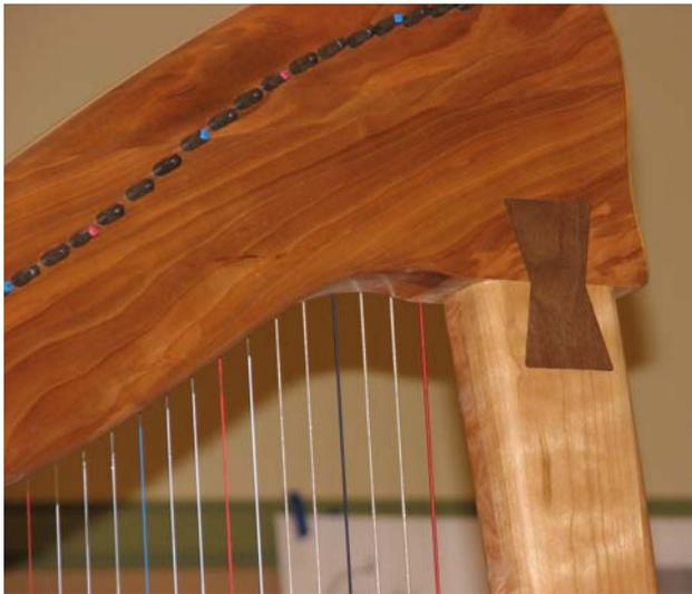
*Joinery detail. The duthman is structural.*
